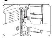
Unlatch the paper guide and open it in the direction of the arrow.
